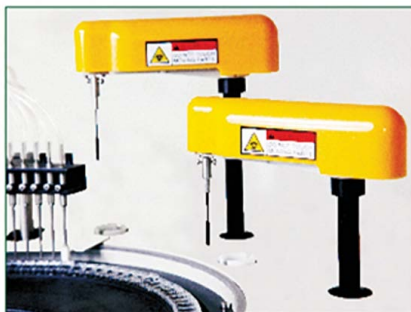
Independent mixer ensuring full reaction of sample / reagent solution.
