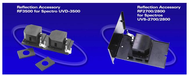
The Reflection Accessory can measure the reflectance spectrum of a solid surface. such as an optical surface, crystal surface, film-coated lens and so on. As reflecting mirror on the reference beam is the "standard reflecting mirror", the user can calculate the absolute reflectivity of the measured surface.
